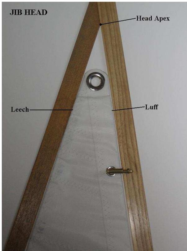
**NOTE:** On the girth measurement, be sure to use the head apex when matching up to the tack and clew. Do not measure cringle to cringle as this will incorrectly increase your girth measurement. Refer to the photos at left and below, 4a-c.
