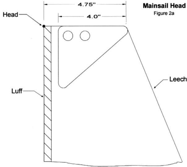
10.2 The mainsail shall contain three battens spaced approximately equally along the leech. The upper batten shall not exceed 15 inches, the middle batten shall not exceed 24 inches, and the lower batten shall not exceed 21 inches.
