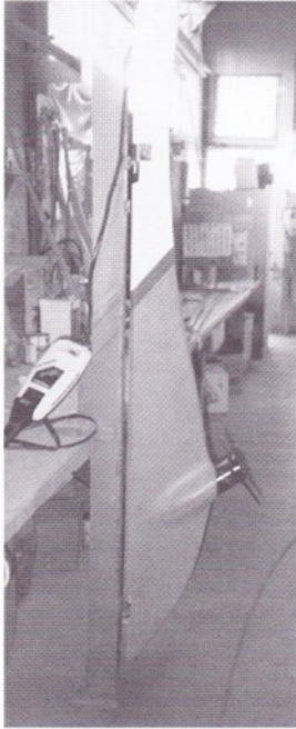
Full view of electric motor and control unit which rests on boat's deck.
